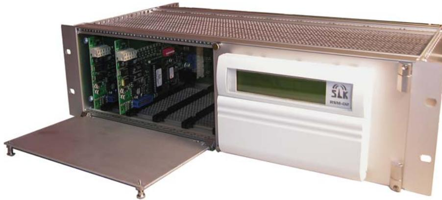
Now there is an alarmreceiver developed in Sweden for nearly all standardprotocols used by the various alarmtransmitters and alarmcentrals on the market. The incoming alarms are exported by a serial interface to a PC for interpretation to plain language of the incoming events.
